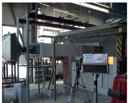
SMOKE EXTRACT DUCT
